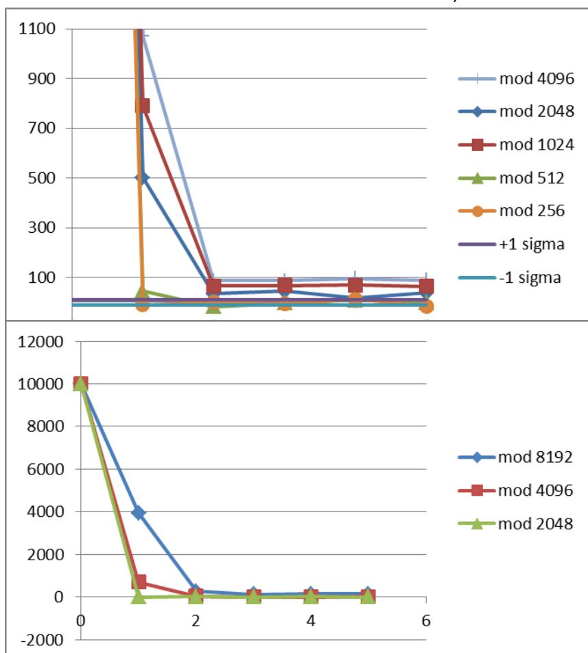
For OSR = 512, the story is much the same. In this case the data were divided by 2 before processing, so the modulus 8192, which here is seen to reduce the correlation at one lag to 0.016, is equivalent to 16384 applied to the raw data. An actual 8192 is shown here as 4096, and reduces that correlation to 0.0018. The limit set by the flatness requirement is here  $m < 9120$ , again more stringent.
