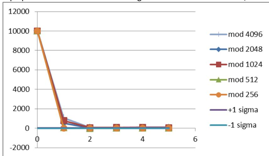
As the modulus decreases, the correlations also decrease. When the modulus is as small as 512, the correlation at one unit lag is only 0.0045, and at modulus 256 the largest correlation magnitude (at lag 5) is -0.0015, or 1.5x the expected standard deviation for these points. Yes, there is a separate limit on the maximum modulus that is set by the need for uncorrelated samples, but one that is not more stringent than the limit  $m < 280$  set by the requirement for a flat distribution.
