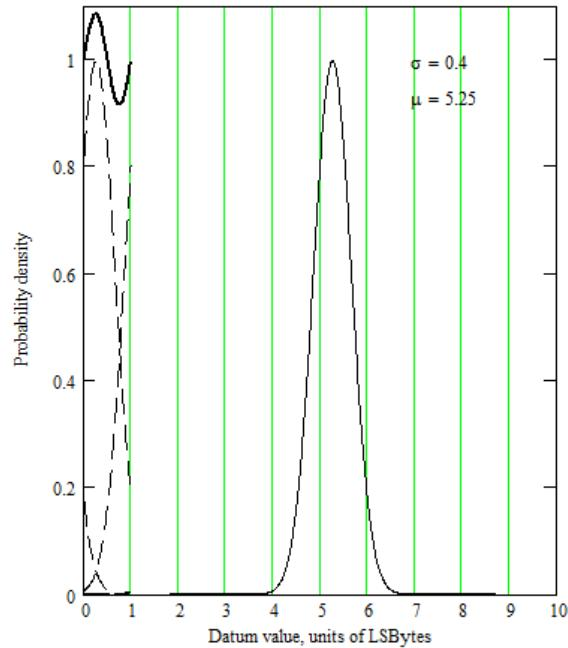
Well, how about adding a little more noise? When the Gaussian is only 20% wider, the variations in the heavy black trace shrink markedly. Let's plot that black trace separately, and follow its behavior as we increase  $\sigma$  (and thereby increase the width of the Gaussian) by a few more steps.
