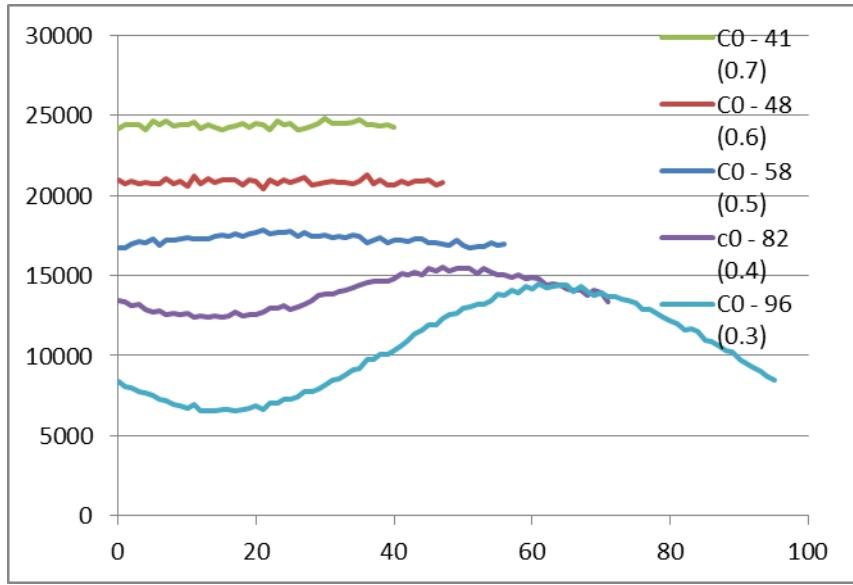
require that the standard deviation be at least 0.7 times the modulus (modulus  $\leq 1.4$  times standard deviation) then we sum together data that are 41 bins apart and get the top green trace. Intermediate values of the modulus give intermediate results, with the total systematic variation decreasing rapidly as the modulus decreases. Towards the top any systematic variation is lost in the natural noise.
