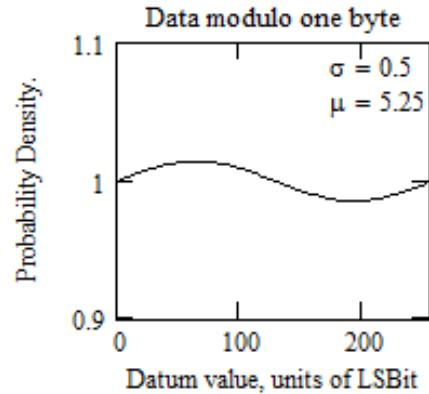
As the standard deviation increases, the probability density rapidly flattens out until its variation becomes completely invisible when plotted at the original scale.
