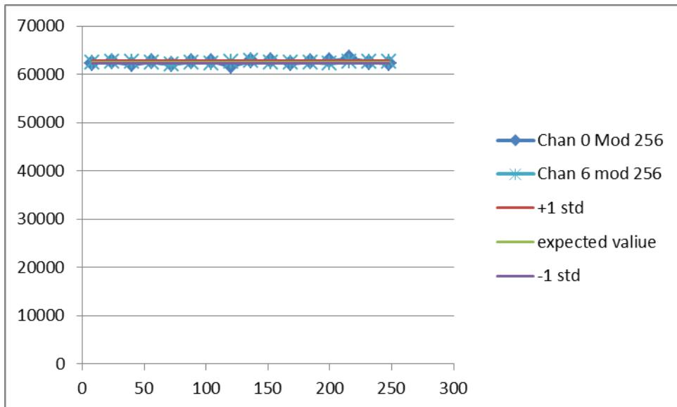
$n+64$  etc. The result is shown in the figure at the right, a satisfactorily flat distribution. The horizontal scale here is in byte values rather than bin numbers. Values on the vertical scale are the contents of the virtual bins summed as above. They represent the bin contents that would have been obtained if the values were first taken modulo 256, and then binned.
