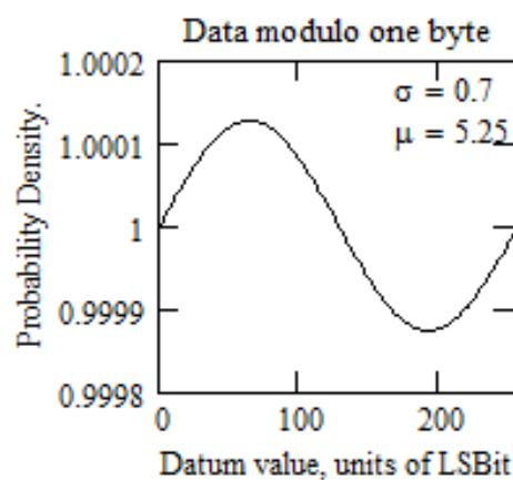
Depending on the needs of a given application, one may choose to work at a variety of positions along this curve, but for sample sizes no larger than  $10^6$ , the criteria  $m \leq 1.4\sigma$  or  $\sigma \geq 0.7m$  would seem to be adequate, in that any systematic deviations from uniformity would be lost in the expected statistical variations in observed frequency. Those criteria are obviously a bit soft and while not quite equivalent they have been used interchangeably in this document.
