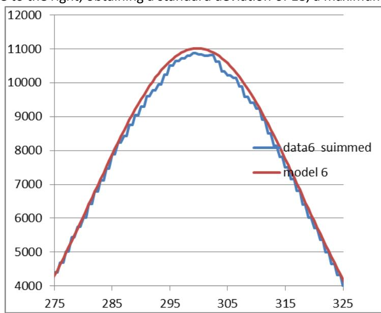
This result, obtained with MSP430f47127 chip 1 is a bit equivocal, because when the same options were set up in chip 2, both channels behaved well with no sign of a preference for even numbers, and gave a standard deviation of 18.5. So at least here it looks like the kind of failure we saw earlier with the byte generator where a few units had the disease, most did not, but the disease affects only some of the possible ways to set up the SD16.
