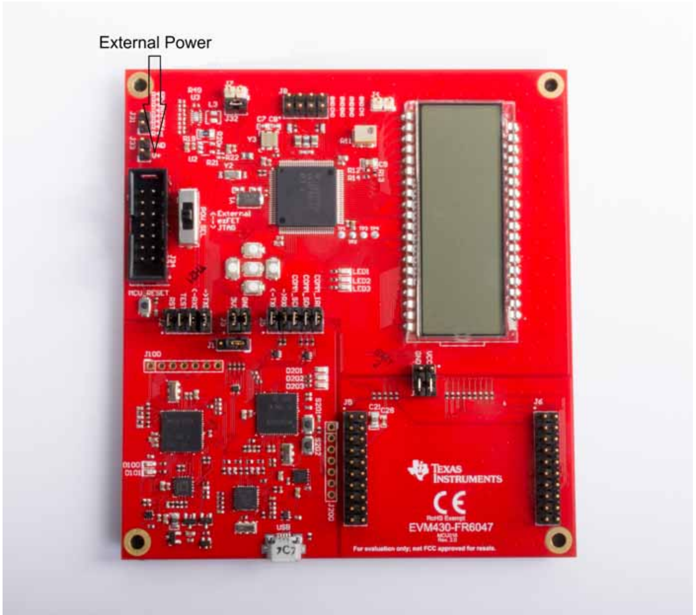
Figure 16. External Power to EVM
