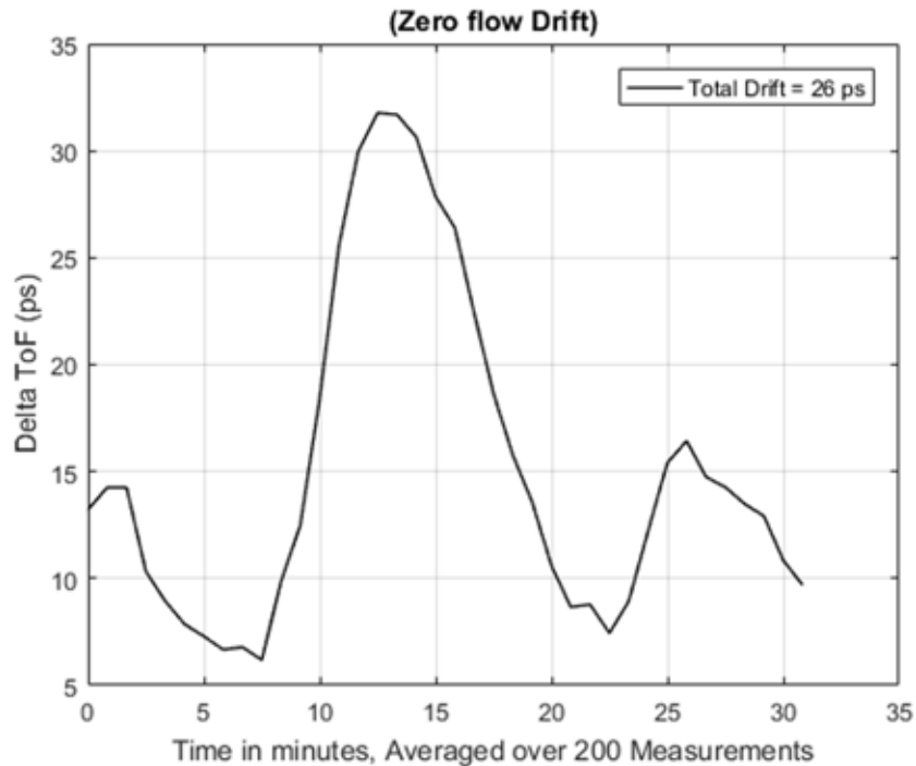
Figure 22. Zero Flow Drift of DToF With Meter In-Oven
