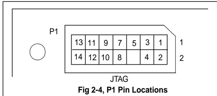
The definition of P1, which has the JTAG signals is shown below.
