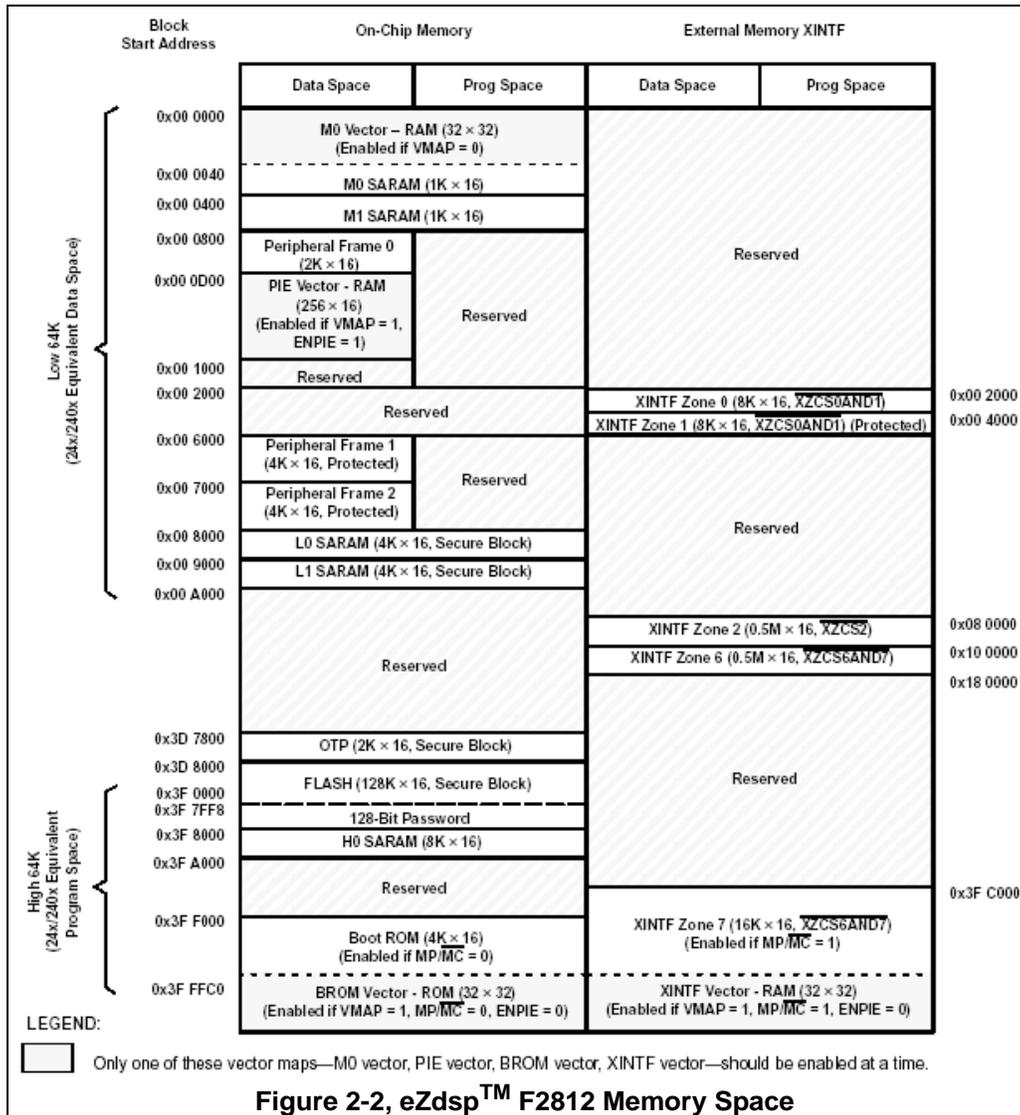
**Note:** The on-chip flash memory has a security key which can prevent visibility when enabled.
