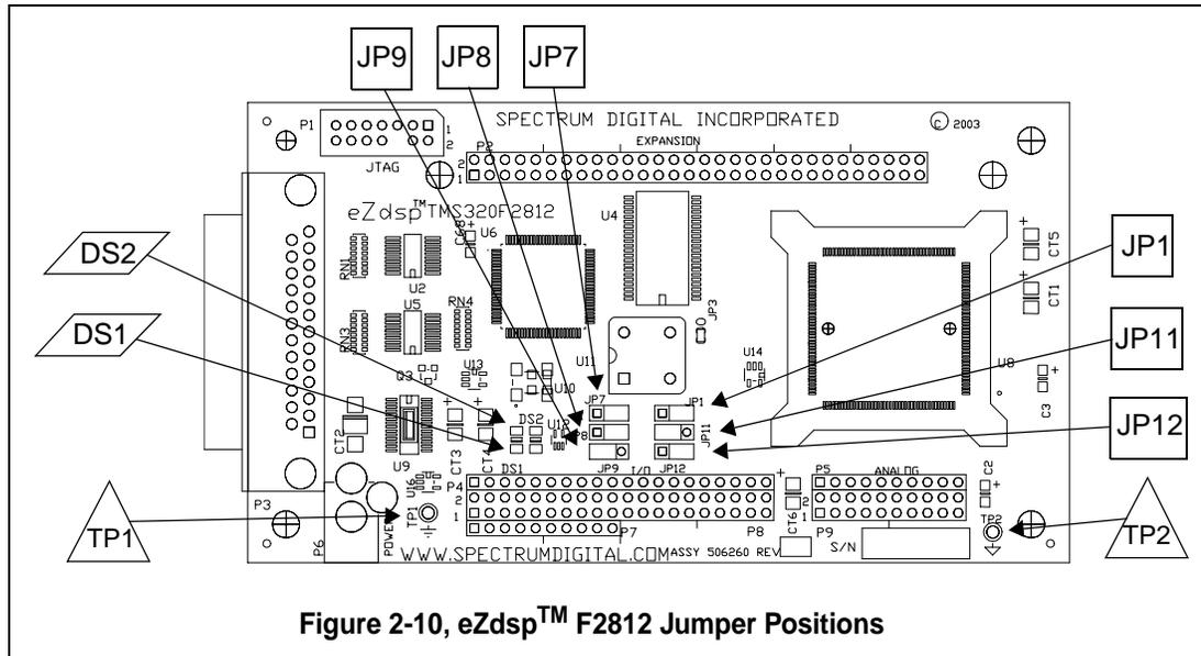
Figure 2-10, eZdsp™ F2812 Jumper Positions
