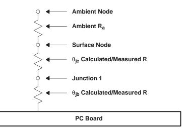
Figure 5. Resistance From Junction-to-Board
