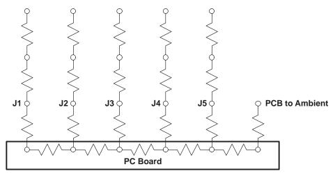
Figure 6. Thermal Conduction Resistances
