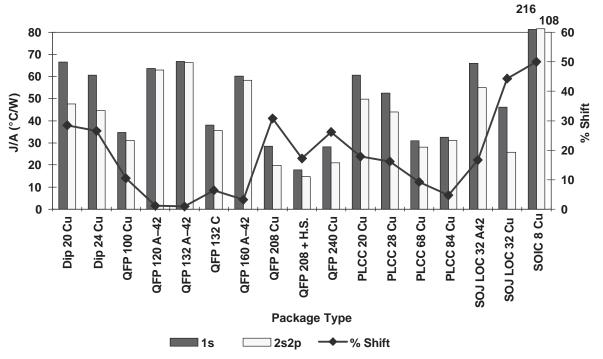
Figure 1. 1s vs. 2s2p PCB for Various Packages
