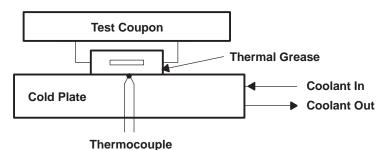
Figure 4. Cu Cold Plate Measurement Process
