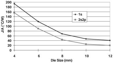
Figure 2. Die Size Impact on a CSP
