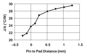
Figure 3. J/A vs. Pin to Pad Distance
