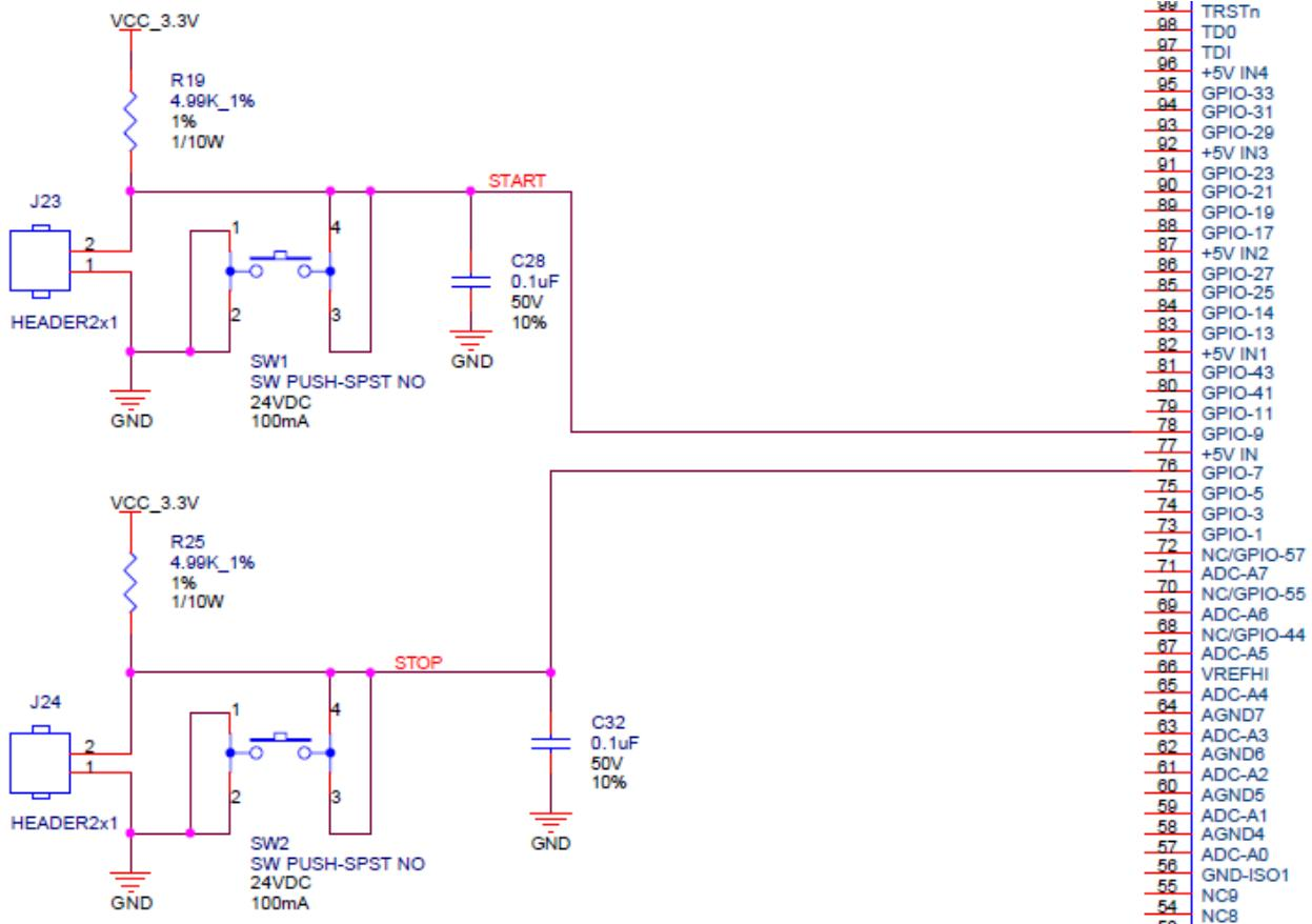
As can be seen, SW2 is connected to GPIO-7 and SW1 is connected to GPIO-9. We need to configure the GPIOs in HAL\_setupGpios() function of hal.c file to allow those pins to be inputs:
