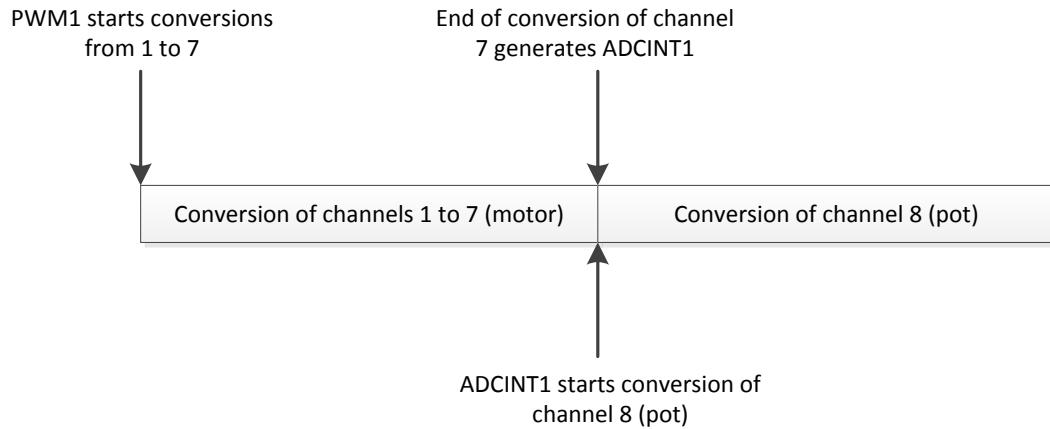
The second change is in hal.h file. A new function is created to read the potentiometer. This function simply reads the ADC result register and scales the value to an IQ24 value. This function is listed here:
