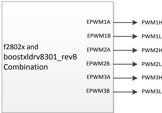
There are two functions that configure the PWM connections. One is in HAL\_setupGpios() to setup the GPIOs as PWM outputs:
