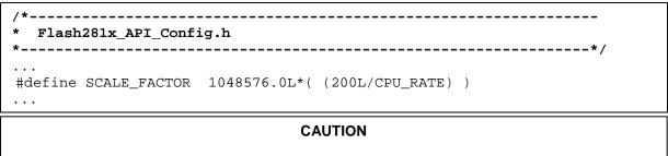
The SCALE\_FACTOR formula is already defined in the file Flash281x\_API\_Config.h. This formula must not be modified. Doing so will cause improper operation of the flash API functions.
