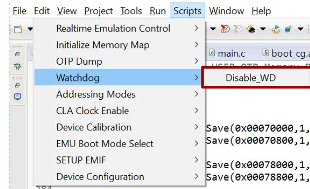
SYS/BIOS can enable/disable the watchdog also. For example for the F2837x devices, the following can be used to disable the watchdog.
