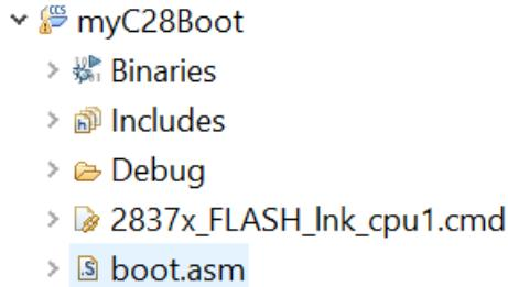
This boot image does **not** use SYS/BIOS. Its purpose is to run first and do “stuff” and then jump into the application’s `_c_int00` function to start the application.
