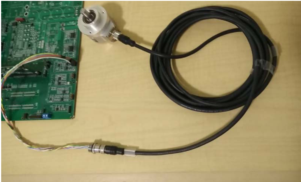
Figure 10. M12 Heidenhain Cable Connects to the Encoder
