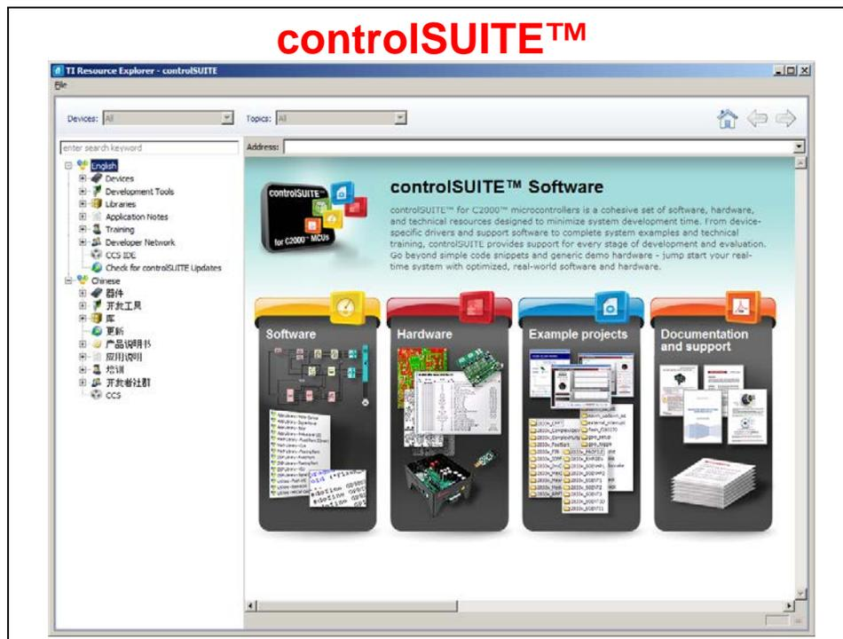
controlSUITE is a single portal for all C2000 software and has been designed to minimize software development time. Included in controlSUITE are device-specific drivers and support software, as well as complete system design examples used in sophisticated applications.
