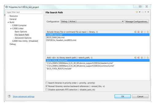
Figure 2.4: Setup Linker Include Paths
