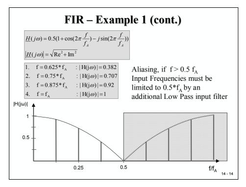
The solution to suppress any frequencies that violate the sampling theorem is to introduce an antialiasing filter before the samples are taken. This way, no frequency component beyond  $f_A/2$  will disturb the digital processing. The anti-alias filter is an analogue low-pass filter.
