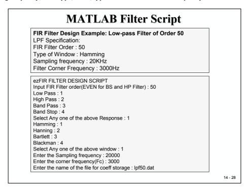
The output of the MATLAB calculation is a list of coefficients and a graph of magnitude and phase of the filter response.
