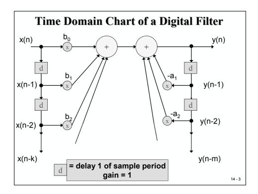
This flow can be used to calculate y(n) from the current input sample x(n) and samples of the input signal, taken one (x(n-1)), two (x(n-2)) or k(x(n-k)) samples before. We call this part the "forward" section of the calculation. If we include the status of the output signal delayed by one period (y(n-1)), two periods (y(n-2)) up to k periods (y(n-k)) into the calculation of the new value of y(n), we add a "feedback" section to the computing scheme.
