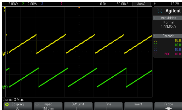
Figure 21 Scope plot of reference angle and rotor position
