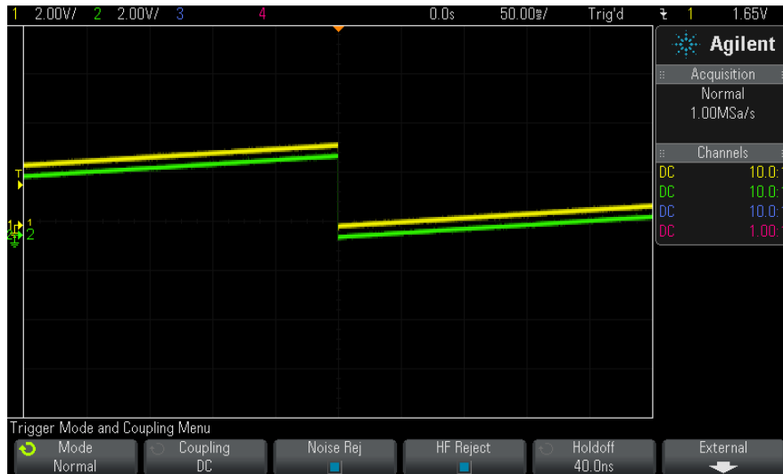
Figure 27 Scope plot of reference position to servo and feedback position
