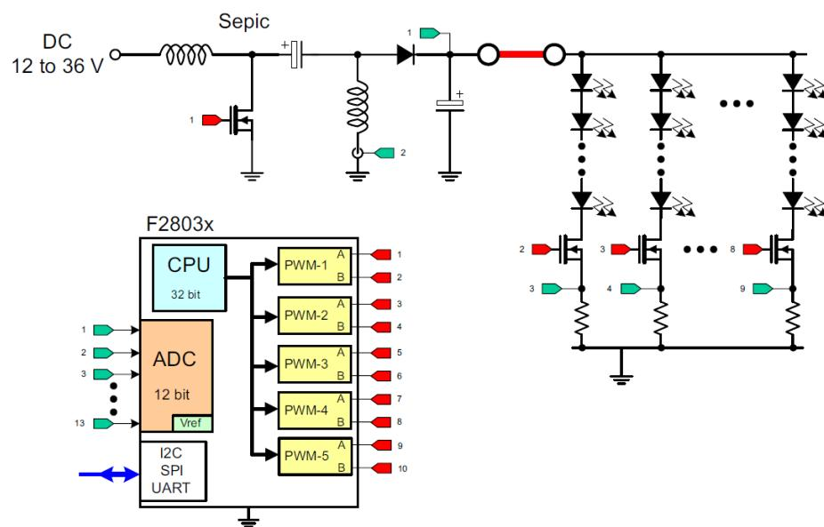
SEPIC MOSFET (red label 1) opens and closes with a frequency that is the **switching frequency**= 100kHz.
