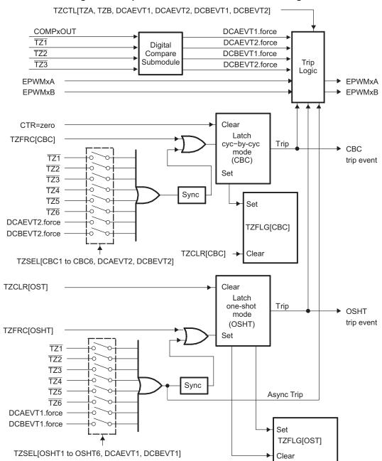
Figure 39. Trip-Zone Submodule Mode Control Logic
