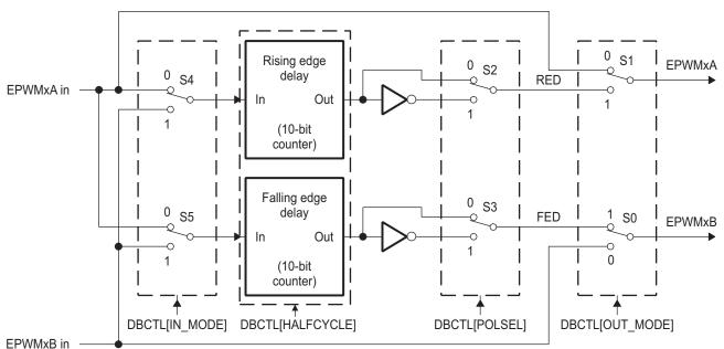
Figure 31. Configuration Options for the Dead-Band Submodule
