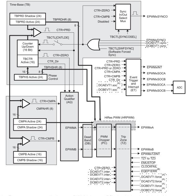
Figure 3. ePWM Submodules and Critical Internal Signal Interconnects
