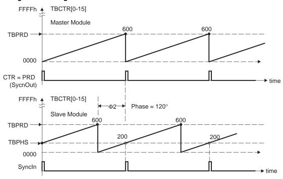
Figure 65. Timing Waveforms Associated With Phase Control Between 2 Modules
