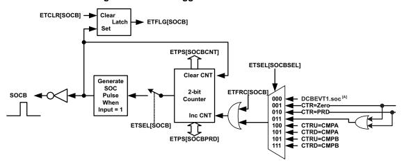
Figure 46. Event-Trigger SOCB Pulse Generator
