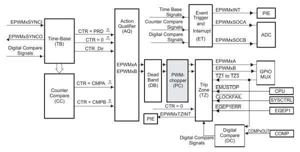
The PWM-chopper submodule allows a high-frequency carrier signal to modulate the PWM waveform generated by the action-qualifier and dead-band submodules. This capability is important if you need pulse transformer-based gate drivers to control the power switching elements.
