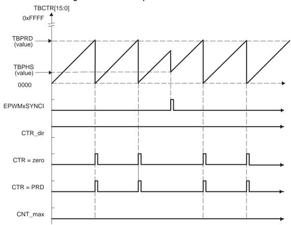
Figure 10. Time-Base Up-Count Mode Waveforms
