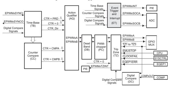
Figure 41. Event-Trigger Submodule
