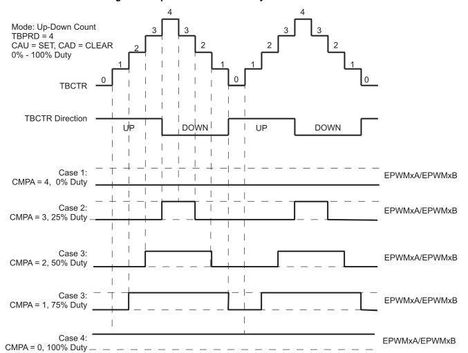
Figure 23. Up-Down-Count Mode Symmetrical Waveform
