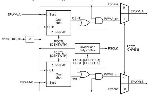
Figure 34. PWM-Chopper Submodule Operational Details
