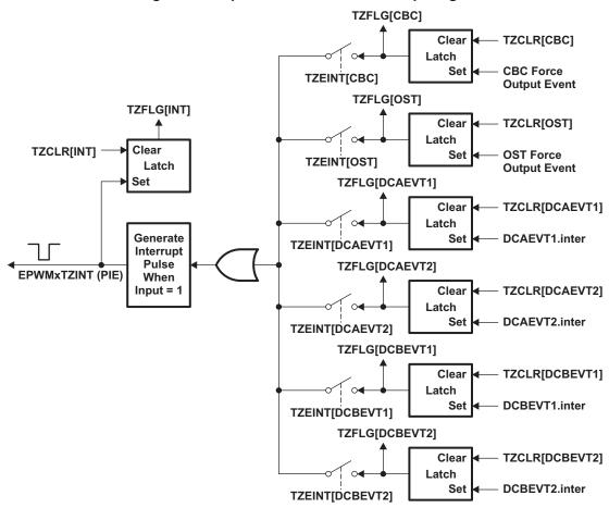
Figure 40. Trip-Zone Submodule Interrupt Logic
