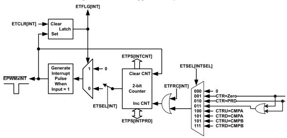
Figure 44. Event-Trigger Interrupt Generator
