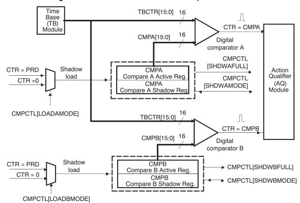
Figure 15. Detailed View of the Counter-Compare Submodule
