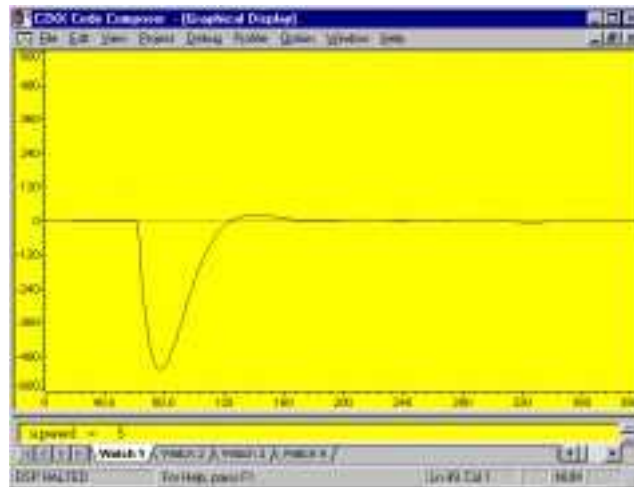
Figure 17. Angular Position Error for a Speed Reversal From -180 rpm to +180 rpm
