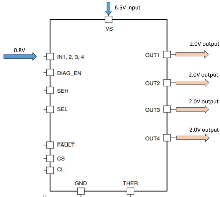
When 0.8 V is input to IN1, IN2, IN3 and IN4, 2.0 V is output from OUT1, OUT2, OUT3 and OUT4.
