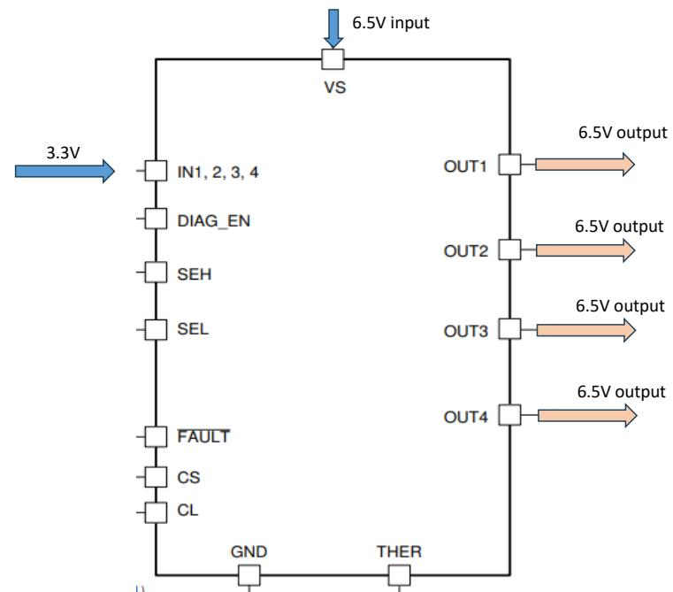
When 3.3 V is input to IN1, IN2, IN3 and IN4, 6.5 V is output from OUT1, OUT2, OUT3 and OUT4.
