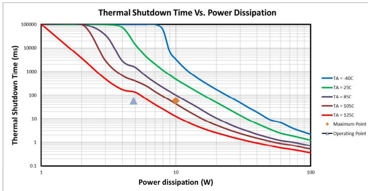
Figure 1: Thermal Shutdown Time (ms) Vs. Power Dissipation (W)
