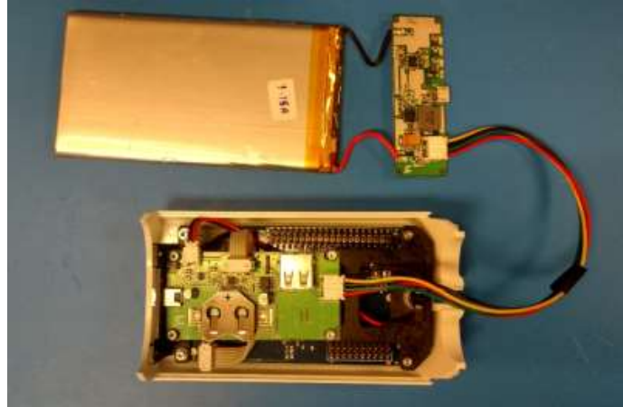
Figure 9. Note the position of 4-way cable.
