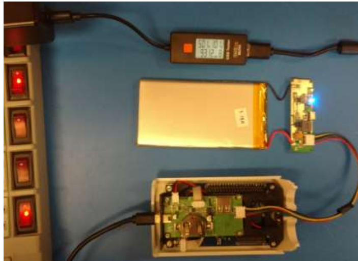
Figure 10. Connections to charge the Battery through Power Controller PCB.
