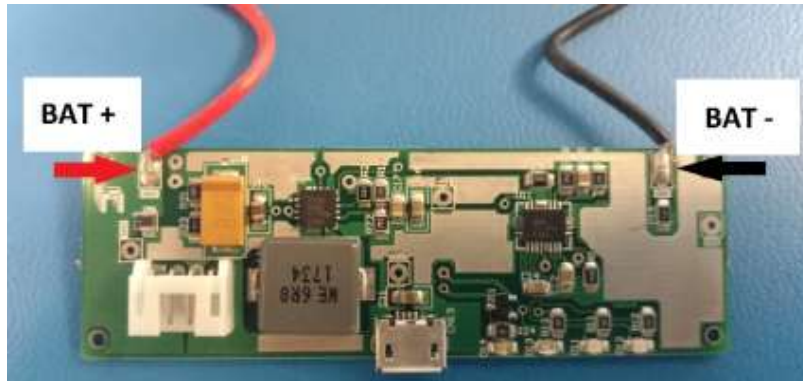
Figure 5. Power and Ground points in Battery PCB
