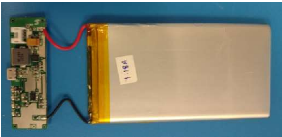
Figure 6. Battery cell soldered to the Battery PCB
