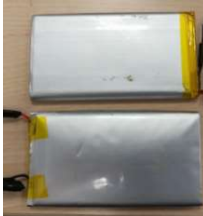
Figure 3. Example of a bad battery cell (on the bottom) and a healthy battery cell (on the top).
