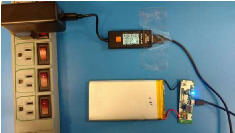
Figure 7. Set up to check Battery PCB charging current from uUSB input.
