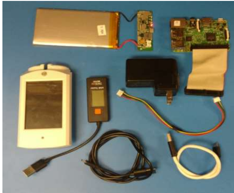
Figure 1. Components and instruments required for PCB QC procedure
