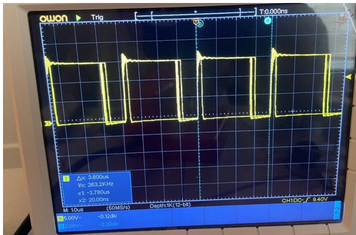
Trace 3) Unstable switch output after scope probe on current limit adjust pin is removed. (subsequently removing scope probe from the switch output for an instant returns the switch output to the stable state shown in Trace 1)
