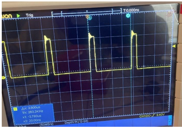
Trace 3) Unstable switch output after scope probe on current limit adjust pin is removed. (subsequently removing scope probe from the switch output for an instant returns the switch output to the stable state shown in Trace 1)
