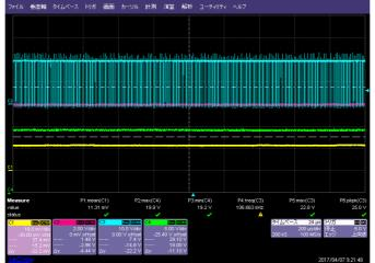
Vin:30V~20V→Waveform is stable.
