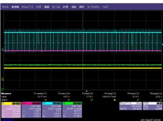
Waveform when the output voltage starts to decrease  $\label{eq:vin=18.1V} \mbox{Vin=18.1V,Vout=17.1V} \rightarrow \mbox{17.00V}$
