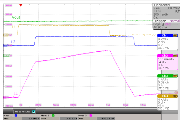
Figure 8-11. Switching Waveforms, Boost Operation
