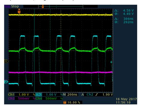
Since the part seems to work fine when the Ferrite bead on the output is shorted it seems that the bead is part of the problem. However even with the bead shorted there is a lot more noise on the output voltage than expected.
