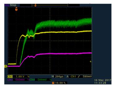
Here are several screen shots at a smaller timebase showing the switching waveform. These two are images taken at startup with various trigger settings to capture different parts of the startup sequence.
