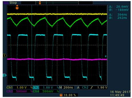
This image is with the output side ferrite bead FB9 shorted with a pair of tweezers. Note that the voltage output is at 1.5V, though still very noisy.
