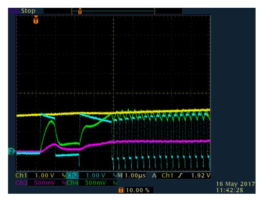
This image shows the Vin sitting at about 4V. There is a lot of noise on the output (Ch4). The feedback voltage has settled to about 800mV whereas it should be 450mV. This is after the supply has settled to steady state. The Vout is measured at the output capacitor, before the ferrite bead.
