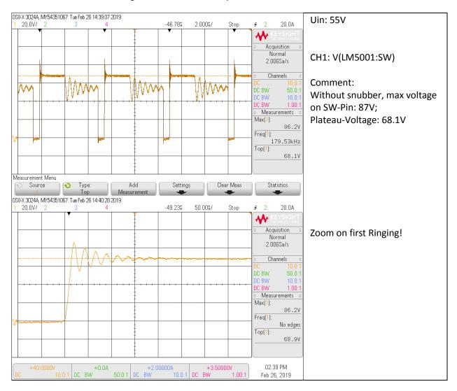
By adding an RCD-Snubber the voltage can be reduced. See following pics.
