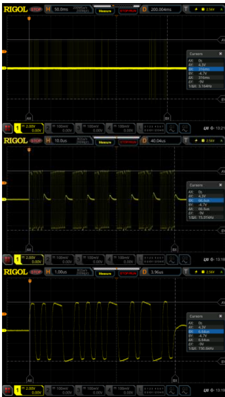
BQ79600EVM + BQ79656EVM, Probing BQ79656EVM J20 (COML after filter/isolation) Wake up
