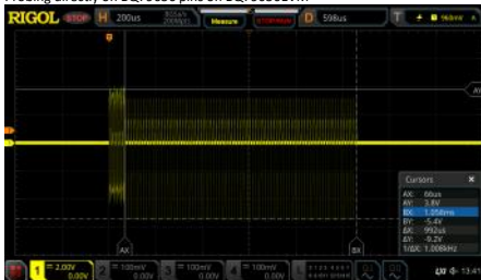
Probing directly on BQ79656 pins on BQ79656EVM
