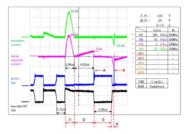
1 The high-side FET turns on and the voltage accumulated in the clamp capacitor flows to the secondary-side rectifying capacit 2 Since the high-side FET is ON as it is, an exciting current flows through the transformer. (Minus side)
