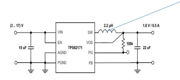
If the inductor's ferrite core breaks down (There is no ferrite part)  $2.2uH \rightarrow 0H$ .
