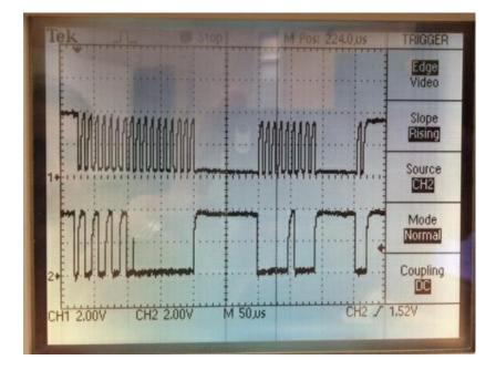
enter I2CCommand 01 Byte 00 press Write Byte button (The scope waveforms occur in this order. AA, 01, 00)
