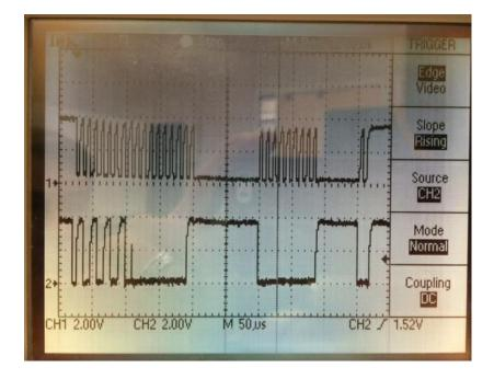
enter I2CCommand 00 press Read Byte button; GUI returns a 04 (The scope waveforms occur in this order. AA, 00, AB, 04)
