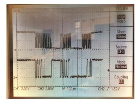
enter I2CCommand 01 press Read Byte button; GUI returns a 08 (The scope waveforms occur in this order. AA, 01, AB, 08)
