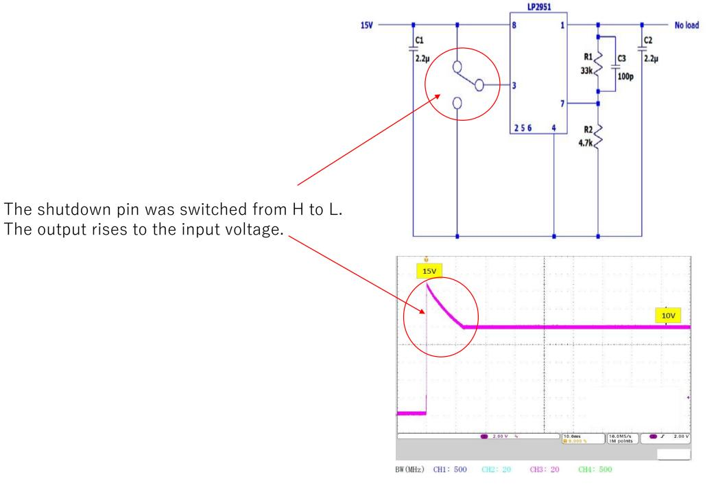
The output rises to the input voltage.
