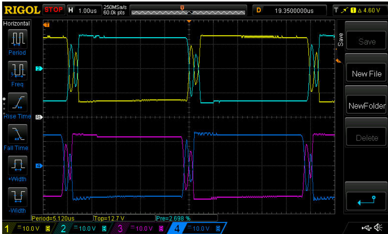
FIGURE 1. UCC28950 GDT Q1-Q2 PA LEG (Yellow, Teal), GDT Q3, Q4 AP LEG (Magenta, Blue)
