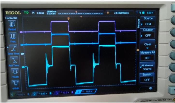
FIGURE A: UCC28950 - BOTTOM Channel 2 - muRata Ps #1002C GDT SEC 1 (Pin #5 & Pin #6) Identical signal on SEC 2
