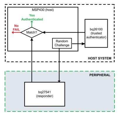
Figure 10. Authentication Scheme (host does not perform authentication transform)
