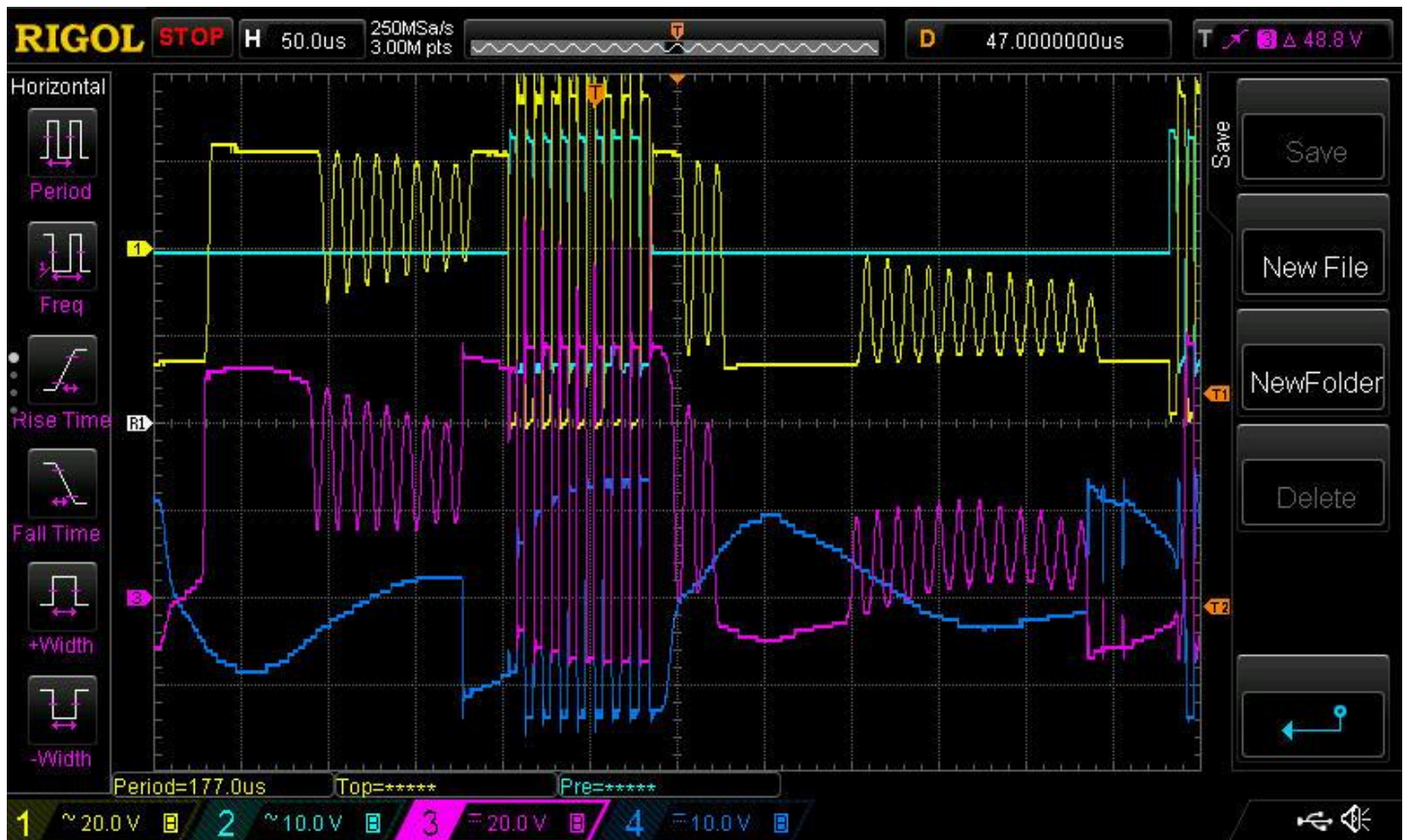
FIGURE 17. TOP WAVEFORM Q1 Q2 GATE, BOTTOM WAVEFORM Q3 Q4 GATE, ROUGHLY 45V DC INK
