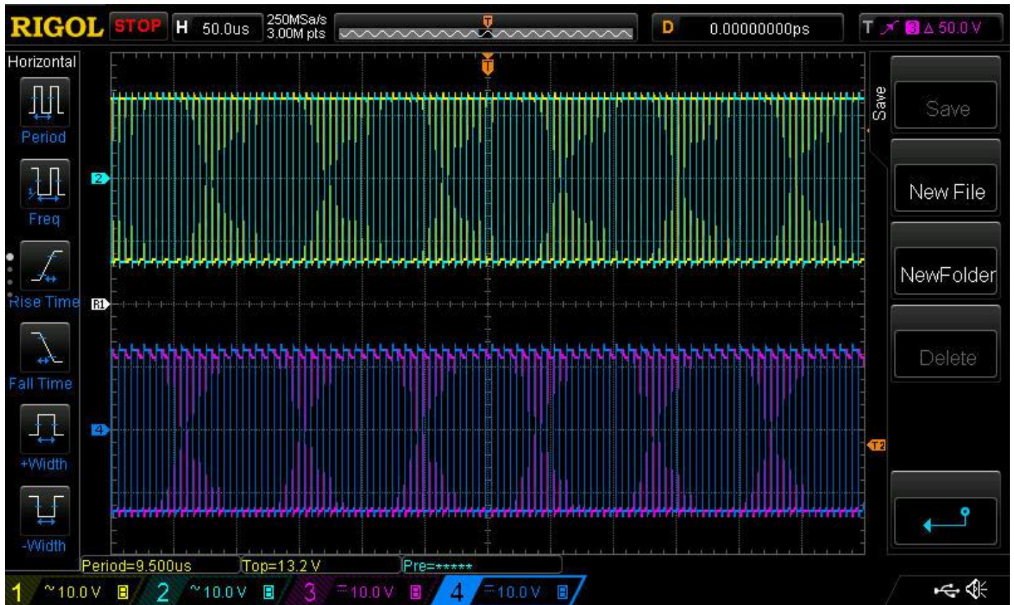
FIGURE 2. TOP WAVEFORM Q1 Q2 AT MOSFET GATE, BOTTOM WAVEFORM Q3 Q4 AT MOSFET GATE NO DC LINK
