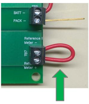
Replace shunt with current meter.
