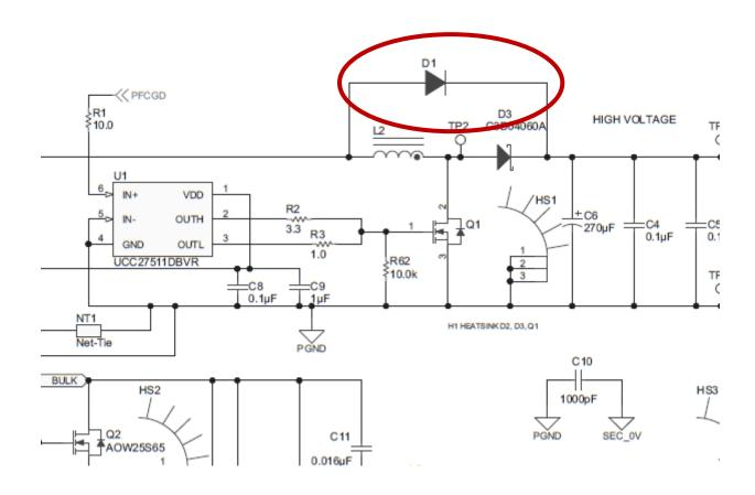
Adding D1 implies Vbulk side expects to see initial instantaneous voltage from AC line to start the controller
