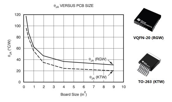
Figure 4.  $R_{\theta JA}$  Vs PCB Size
