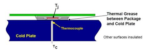
Figure 5. R<sub>e.IC</sub> Measurement
