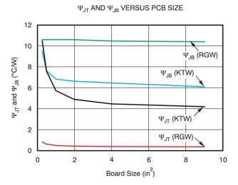
Figure 8. Ψ Versus PCB Size
