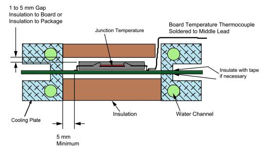
Figure 6. R<sub>BJB</sub> Measurement
