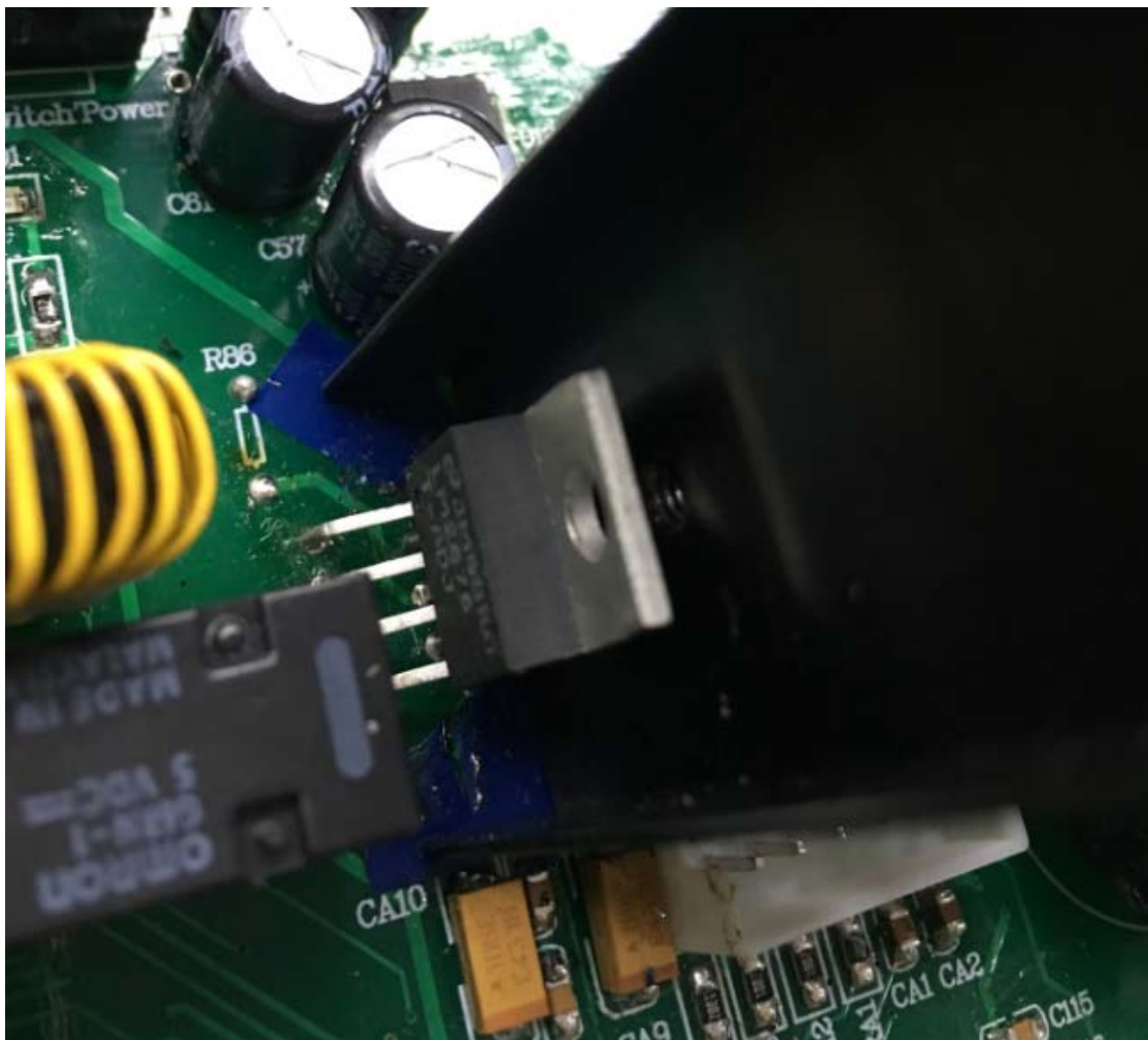
Fig 2.2 LM2676 without heatsink
