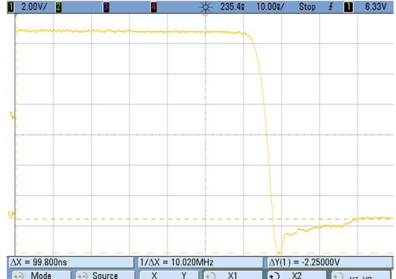
bq25895 12Vin 4A charging with snubber
