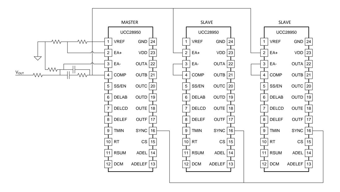
If you have two <u>UCC28950</u> power converters operating in parallel using peak current mode control with one feedback loop they should share current fairly well. The configuration you sent looks correct.
