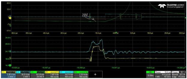
This should be illegal by the controller and is quite dangerous for the input capacitors. I'm also guessing that at this moment the current emulation isn't working as intended.
