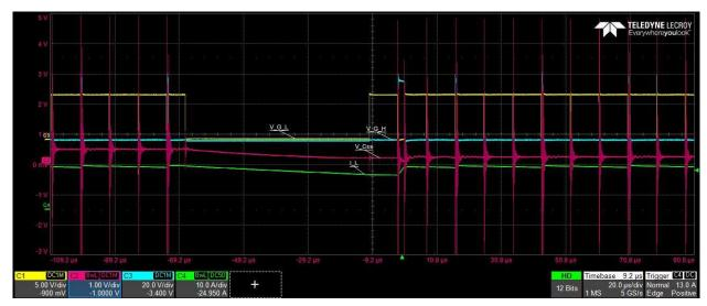
Here I added the voltage at the SS pin to show that the controller indeed shorts the capacitor to restart the hiccup cycle with a soft start, here it is when it wakes up without soft start:
