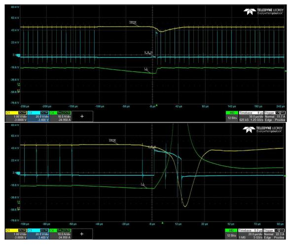
In both cases the error output doesn't seem to discharge very fast or very low so it is plausible that the converter wakes up very violently.
