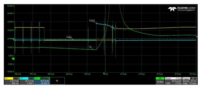
Here you can see the high side gate, low side gate, and the inductor current.
