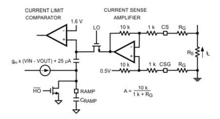
Because of the very short LO switch cycles, it may be possible that we are working with a very dangerous timing with the upper capacitor that should charge to (IL\*Rs\*10) + 0.5V but if the switching time is very short and charge-enable switch has high resistance then maybe the emulated valley current is not getting high enough, this wont let the inductor current trip the 1.6V threshold.
