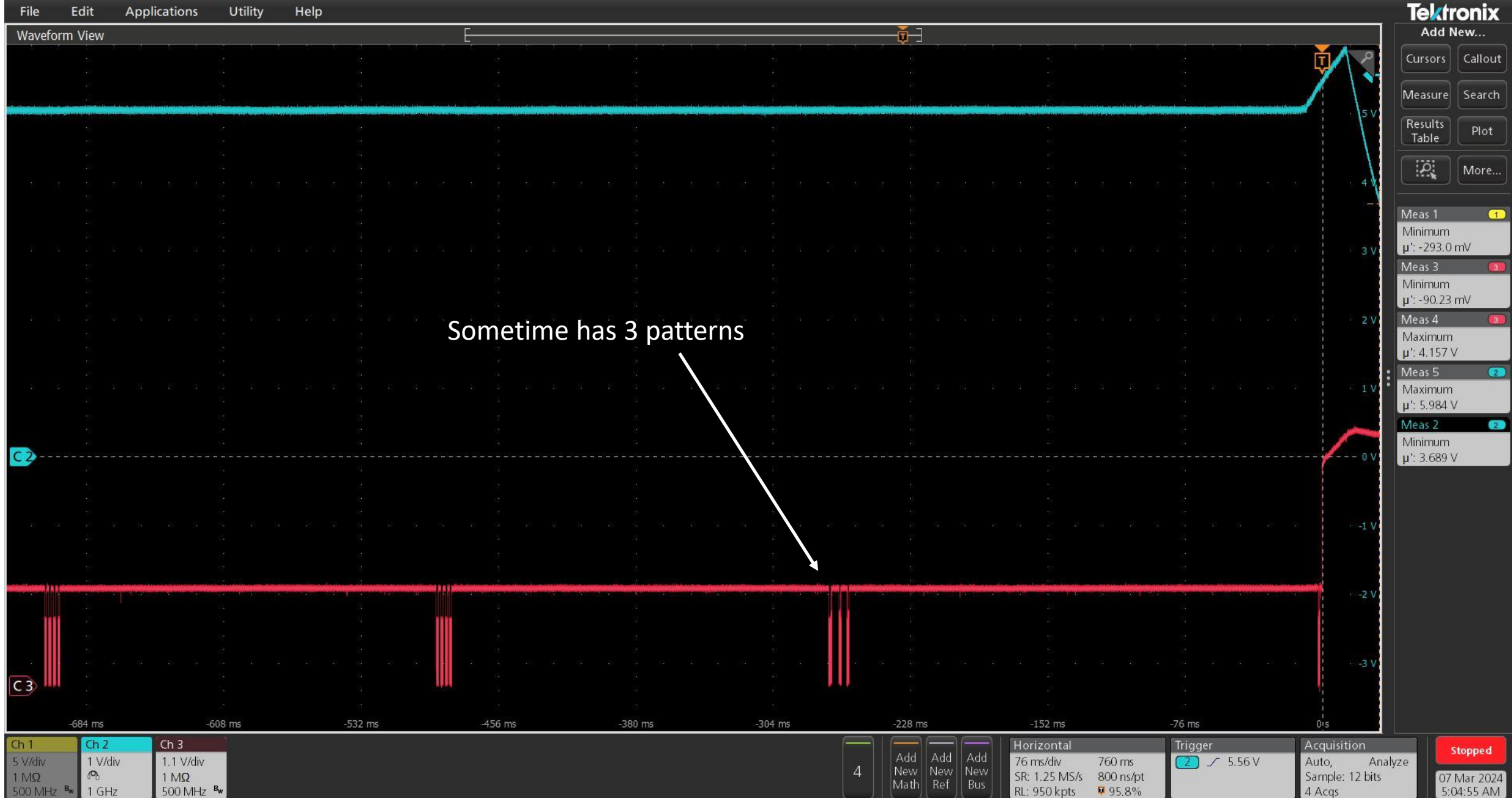
Fig. 04 CH2: Vbus; CH3:CC2;
