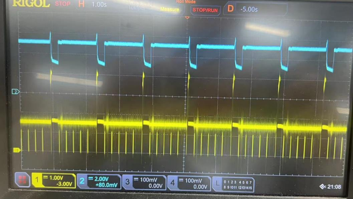
Fig. 01 CH1: Vbus; CH2:CC2;
