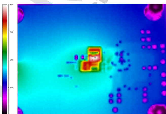
Figure 11. Thermal Image PCB Bottom Side
