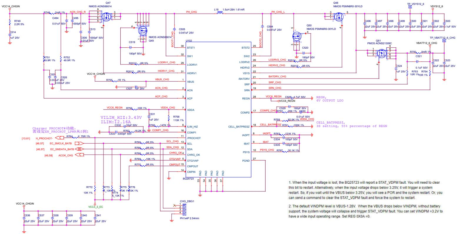
1. When the input voltage is lost, the BQ25723 will report a STAT\_VDPM fault. You will need to clear this bit to restart. Alternatively, when the input voltage drops below 3.25V, it will trigger a system restart. So, if you wait until the VBUS below 3.25V, you will see a POR and the system restart. Or, you can send a command to clear the STAT\_VDPM fault and force the system to restart.
