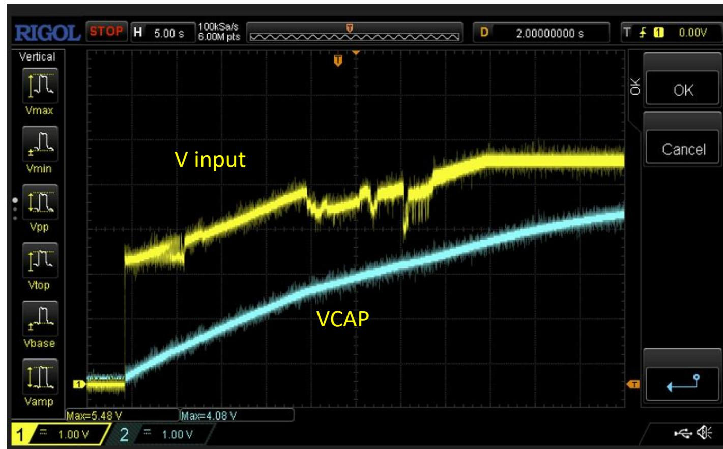
startup waveforms of the input voltages and output voltage in unit with anomaly
