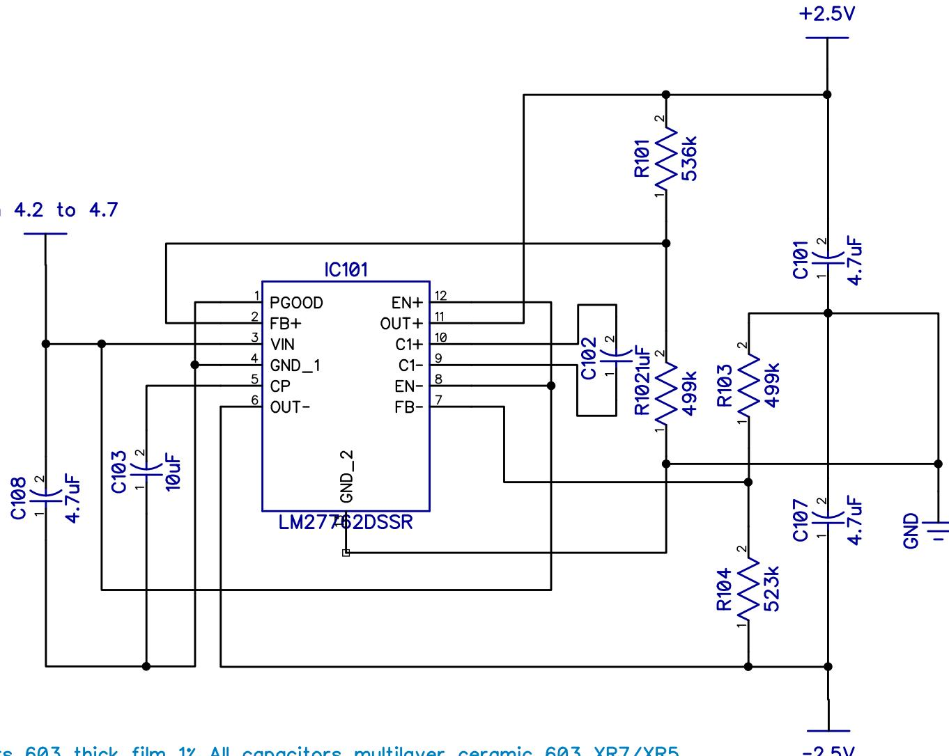
All resistors 603 thick film 1% All capacitors multilayer ceramic 603 XR7/XR5
