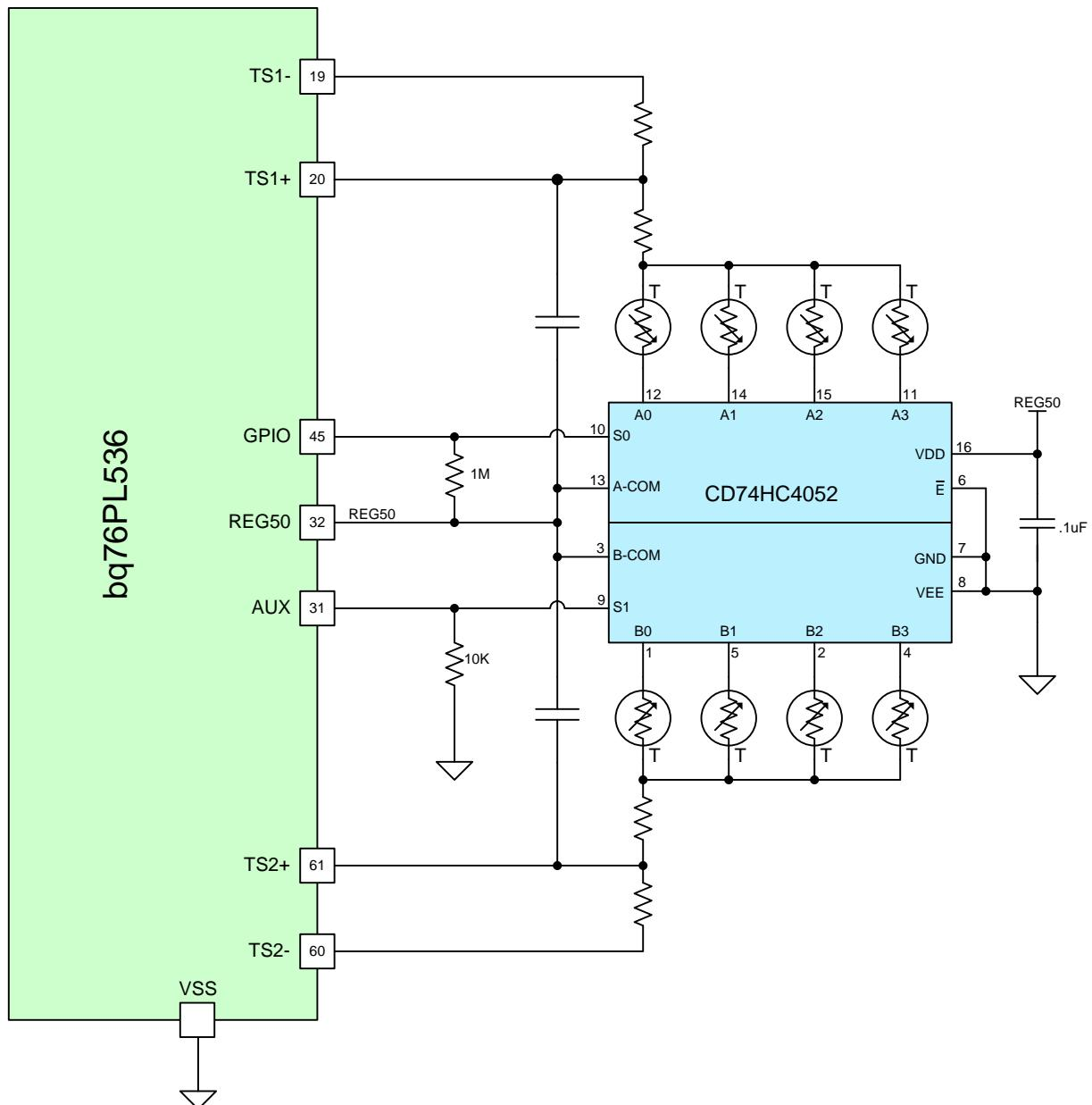
The AUX and GPIO outputs are used to create a 4-state code that controls a '4052 dual 4:1 multiplexer. The mux inputs are connected to 5V (REG50). The 0-1-2-3 outputs are enabled in turn by changing the code to power on a single thermistor to each TS input. Two temperatures are returned on each conversion cycle.
