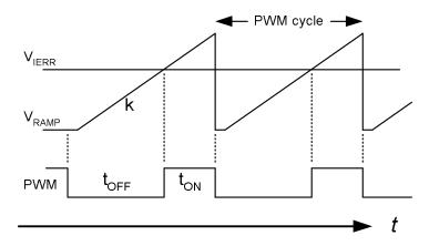
We see that:  $V_{IERR} = k * t_{OFF} = k * T_{SW} * (V_{PK} / V_{OUT}) * |sin(wt)|$
