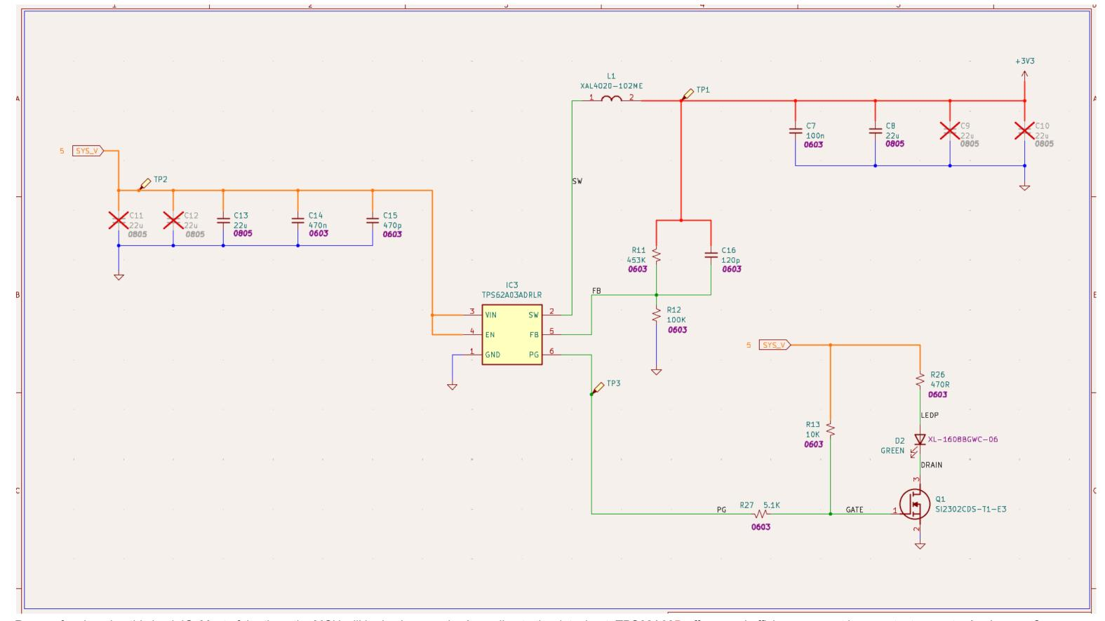
Reason for choosing this buck IC: Most of the time, the MCU will be in sleep mode. According to the datasheet, TPS62A03D offers good efficiency even at lower output currents. Am I correct? Link: <a href="Datasheet Page 12 Figure 8-5">Datasheet Page 12 Figure 8-5</a>. 3.3V Output Efficiency (TPS62A03)
