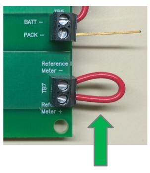
Replace shunt with current meter.
