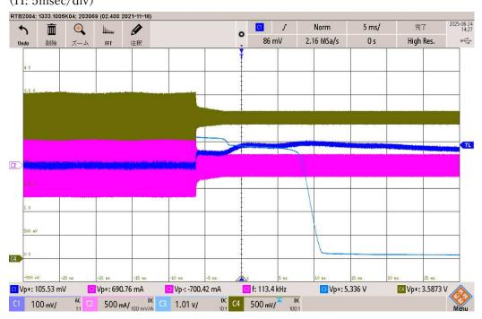
C1: 5Vout [100mV/div], C2: T1 primary current [500mA/div], C3: FB pin voltage [1.01V/div], C4: VCR pin voltage [0.5V/div] (DC mode)
