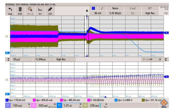
C1: 5Vout [100mV/div], C2: T1 primary current [500mA/div], C3: FB pin voltage [1.01V/div], C4: VCR pin voltage [200mV/div] (AC mode)
