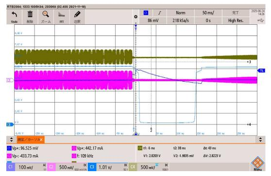
C1: 5Vout [100mV/div], C2: T1 primary current [500mA/div], C3: FB pin voltage [1.01V/div], C4: VCR pin voltage [0.5V/div] (DC mode)
