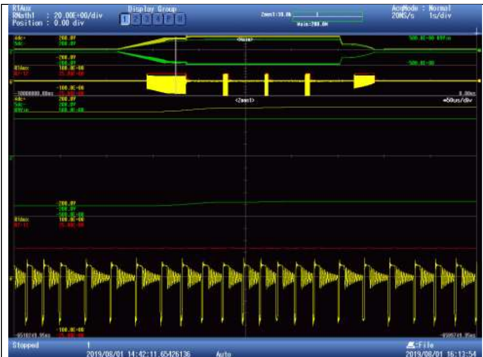
Zoom of above in non-boosting section showing Vout and Vaux operate normally
