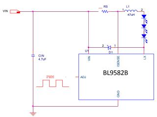
PWM dimming provides reduced brightness by modulating the LED's forward current between 0% and 100%.
